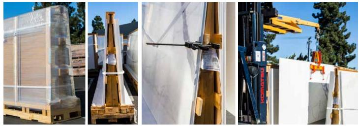
• Use a forklift boom & pitch clamp to carefully move the panels from the original slim factory A-frame, to an A-frame with a wider base and more obtuse angle. We recommend padding the A-frame prior to placing the panels on to each of its sides.
