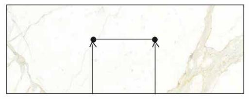
When cutting an "L", drill relief holes where the cut lines intersect, always make the shortest cut first.
