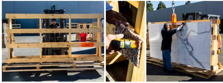
• Use 3 straps to tie the panels to the A-frame, and wrap plastic around the entire A-frame 3X to prepare the package for shipment.
