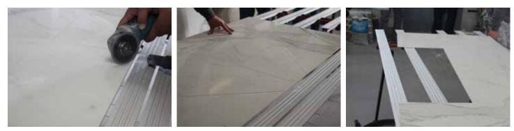
• When manipulating large porcelain panels, a variable speed right angle grinder is strongly suggested to reduce vibration. Electroplated diamond blades or electroplated diamond drill bits should be used for various cuts and manipulations.
