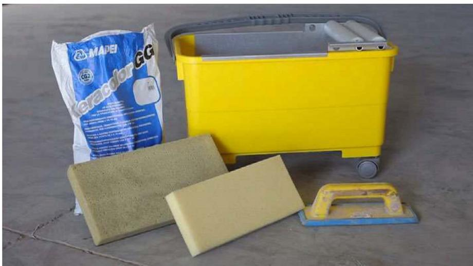
Make the product into a paste by adding water, mixing 5kg of powdered cement with 1.2/1.SL of clean water with a mechanical agitator, until you obtain a smooth paste.
